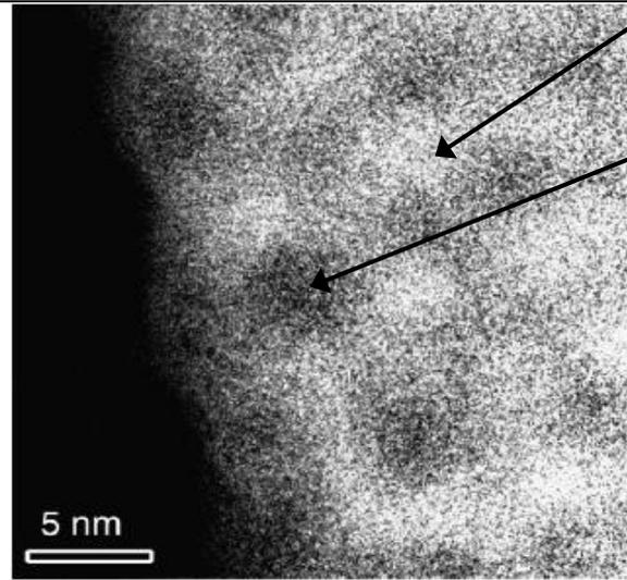
Fig. 8. Distribution map of oxygen in silicon monoxide (multi-window method). Brightness correlates with O content.
