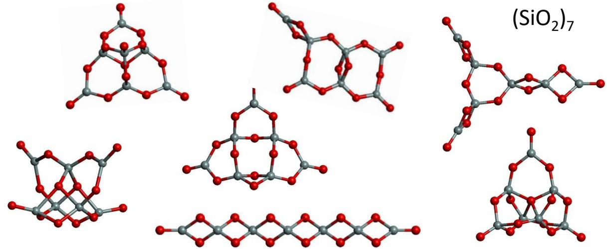
**Complexity:** isomer energy depends on coordinates of all atoms  $E(r_1, r_2, r_3, \dots, r_N)$  leads to a multi-dimensional “energy landscape”
