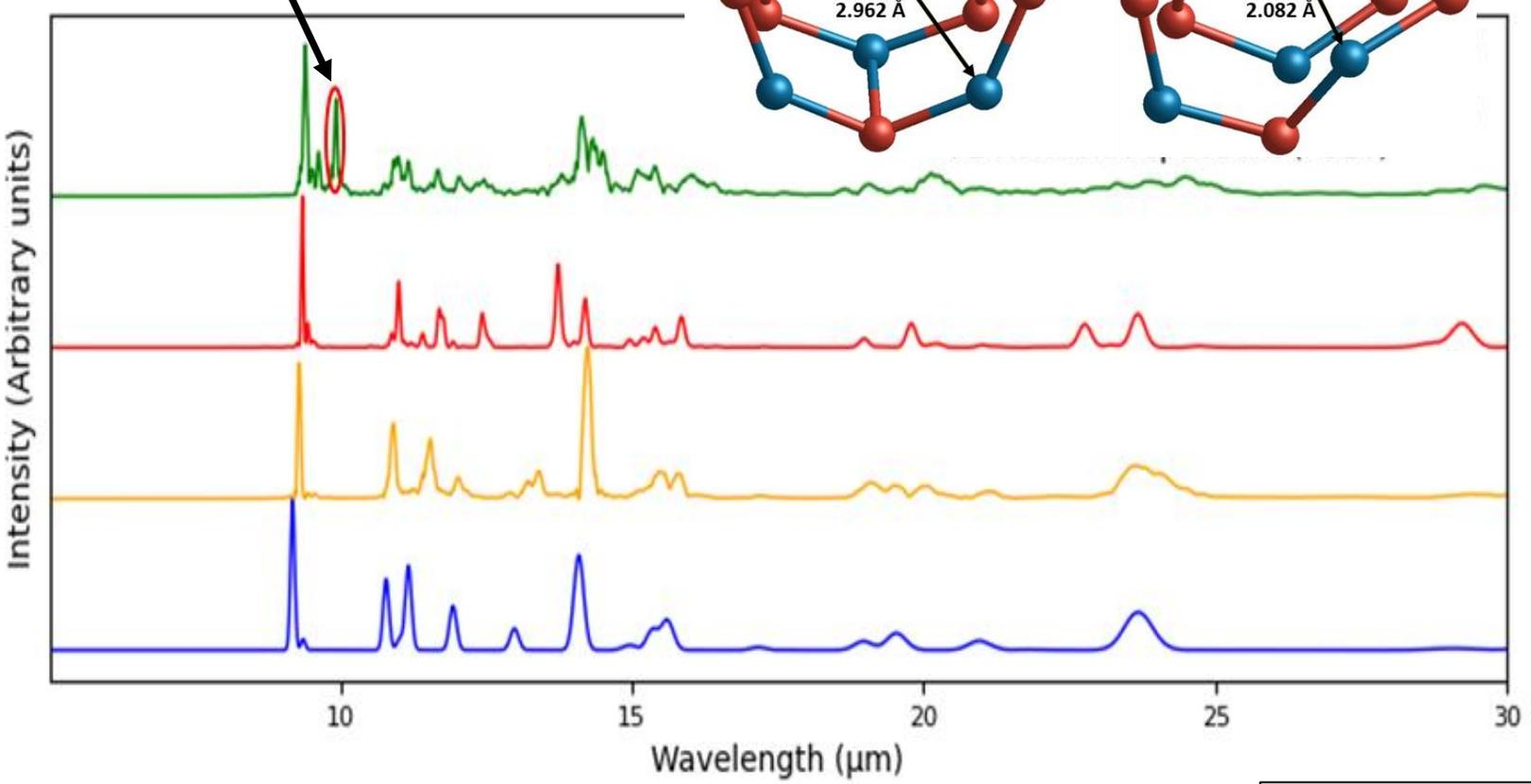
Most features captured by 0K harmonic calculations with some anharmonicity at moderate temperatures
