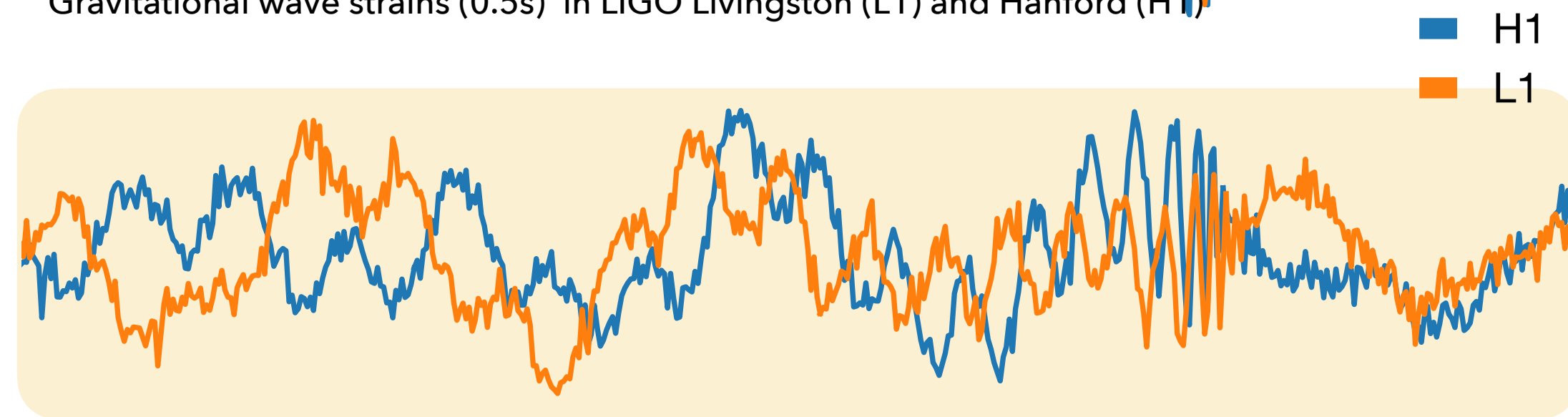
Gravitational wave strains with noises (0.5s) in LIGO Livingston (L1) and Hanford (H1)
